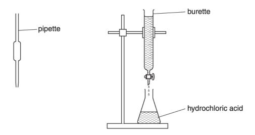
He uses the pipette to measure 25.0 cm<sup>3</sup> of hydrochloric acid into the flask.
