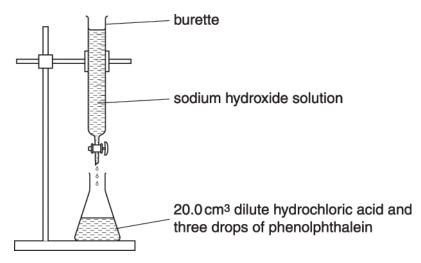
Brian adds sodium hydroxide solution slowly until the phenolphthalein changes colour. He does the titration four times.
