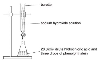
Brian adds sodium hydroxide solution slowly until the phenolphthalein changes colour.
