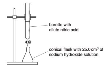
Sam adds five drops of litmus indicator to the conical flask.
